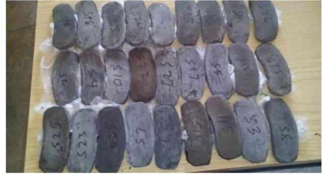
Fig. 2. Heat treated Seashell Reinforced Brake pad Samples.
