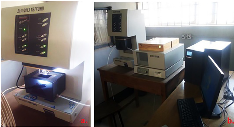
Fig. 1. The Dynamic Mechanical Analyzer and Testing Set up.
