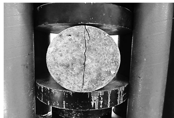
Fig. 19. Mode of Failure and Crack Pattern of HSC Specimens with 0.6 Fiber Percentage.
