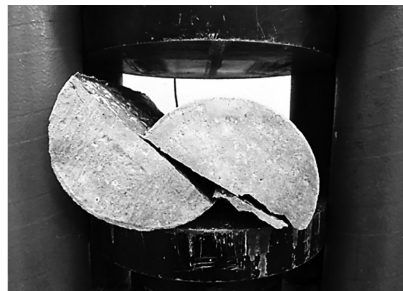
Fig. 18. Mode of Failure of HSC Specimens with 0.3 Fiber Percentage.
