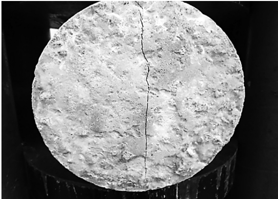
Fig. 20. Mode of Failure and Crack Pattern of HSC Specimens with 0.9 Fiber Percentage.
