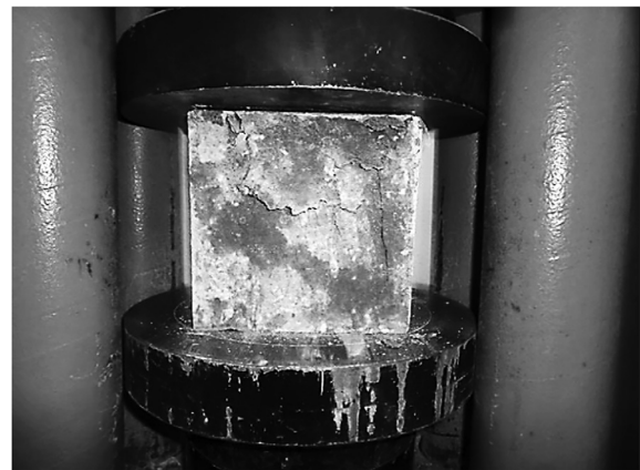
Fig. 11. Mode of Failure and Crack Pattern of HSC Specimens with 0.6 Fiber Percentage.
