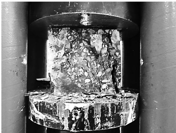
Fig. 9. Mode of Failure and Crack Pattern of Plain HSC Specimens (Without Fiber).
