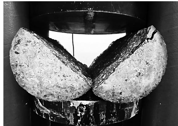
Fig. 17. Mode of Failure of Plain HSC Specimens (Without Fiber).
