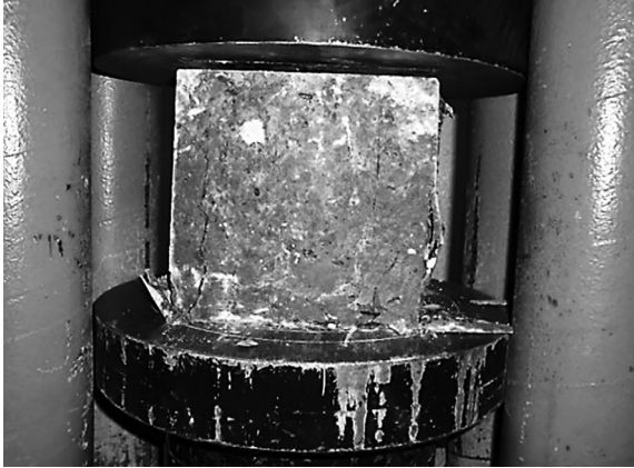
Fig. 12. Mode of Failure and Crack Pattern of HSC Specimens with 0.9 Fiber Percentage.
