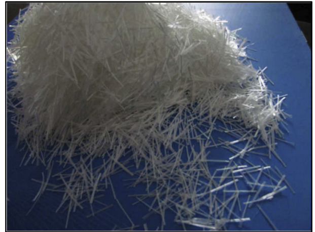
Fig. 2. CEM-FILL Anticrack High Dispersion, Alkali Resistance Glass Fibre.
