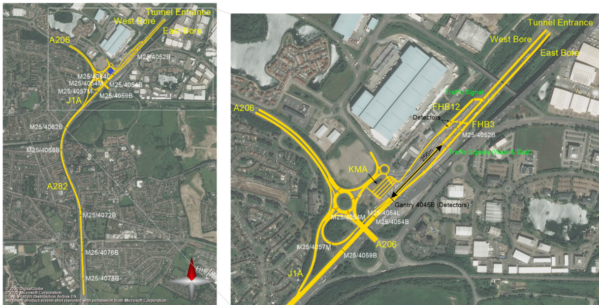
Fig. 1. PTV Vissim model highlighting key roads, detectors, and traffic signal locations at the Dartford Crossing.
