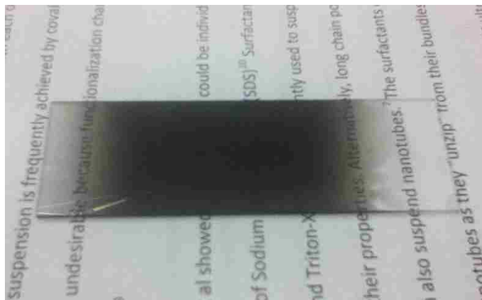
Figure 5: Film of single walled nanotubes sprayed from NMP onto a 3" glass slide. The spray area was 1.5 inches wide, and was covered by repeatedly rastering over the area in 6 sweeps that were 0.25 inches apart. The film is thick enough to be black in the spray area, but becomes transparent as it thins near the edges.
