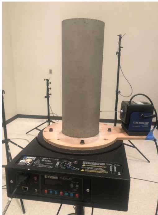
Figure 2-7: Setup of a mounted cylinder on a turntable with a shaker to excite the cylinder. The microphones and reverberation chamber used for ISO 3741 are seen in the background.
