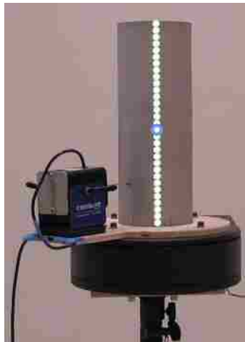
Figure 2-8: Example of one of the 36 line scans taken over the surface of the cylinder to measure complex surface velocities.
