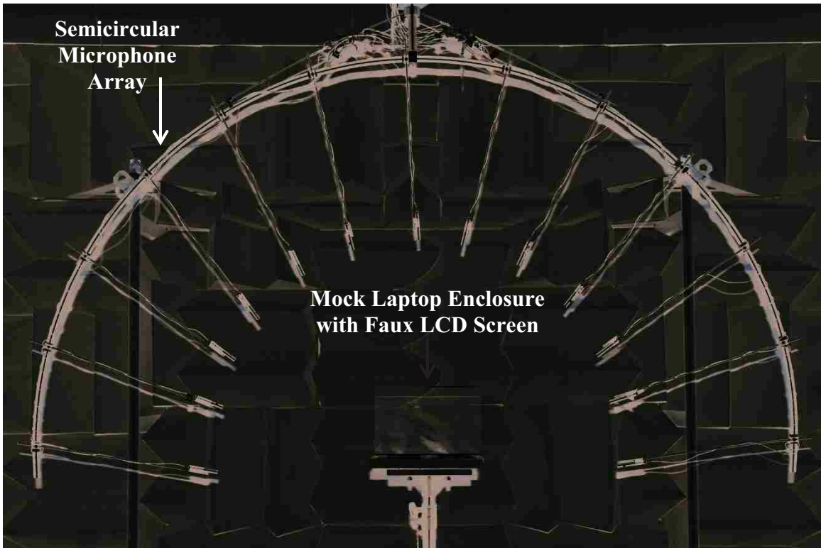
Figure 4-3 – Picture showing the mock laptop enclosure pictured in Fig. 4-2 placed beneath the semicircular array of microphones (56 cm radius).
