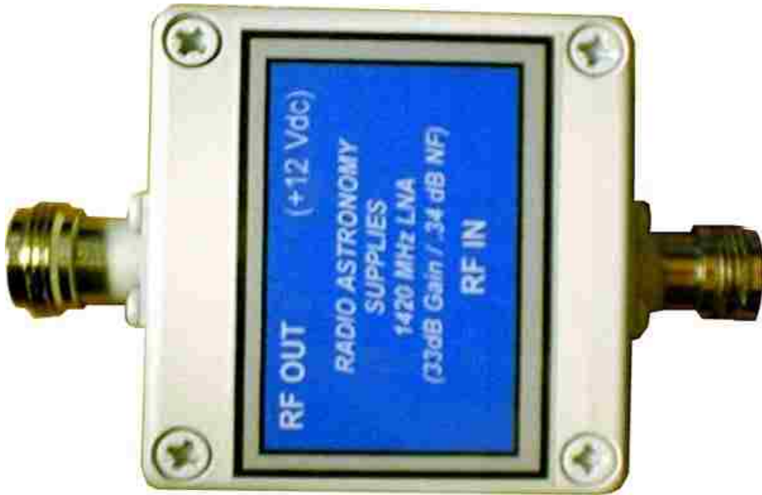
Figure 4-3: Radio Astronomy Supplies 1420 MHz LNA, having 33 dB gain at 0.34 dBm noise figure. Design by Tommy Henderson, WD5AGO.
