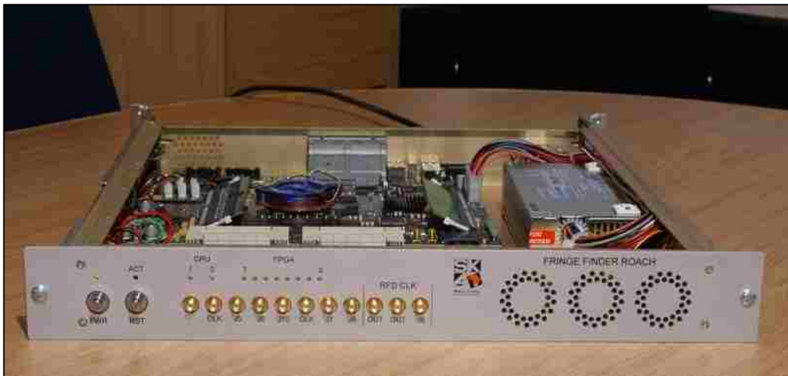
Figure 5-8: CASPER ROACH Hardware, shown in rack-mount enclosure with high-speed A/Ds.
