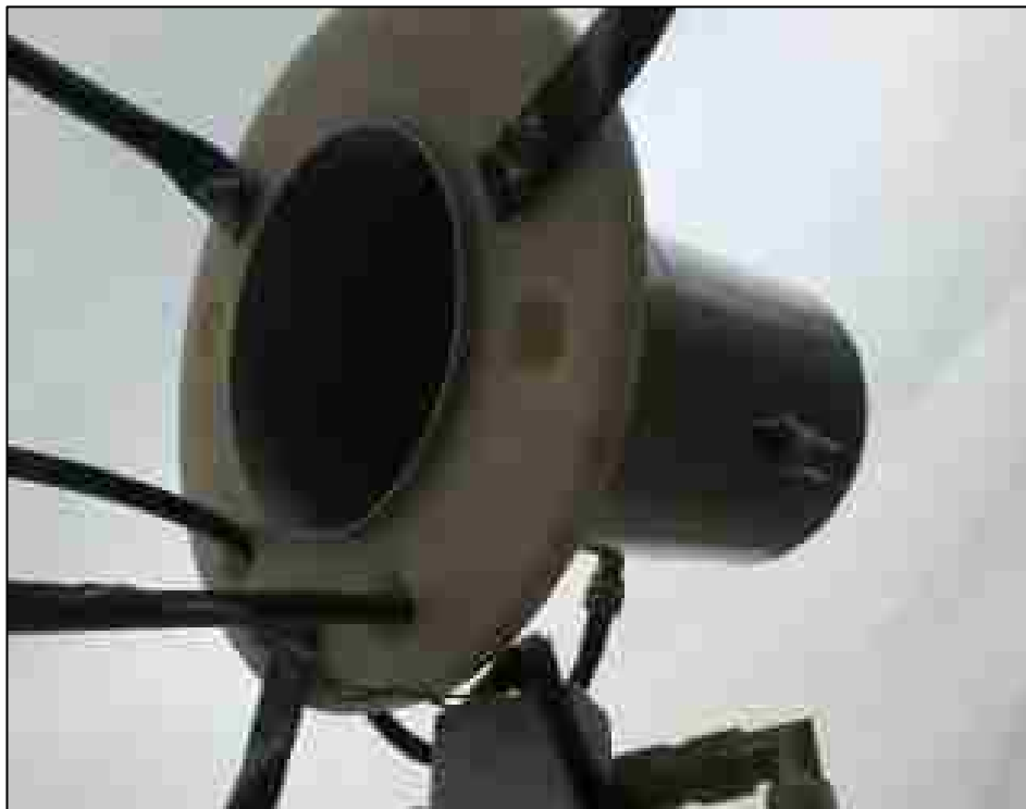
Figure 3-11 The resonator cavity (or can) located at the focal point of the antenna. Photo courtesy of the author.
