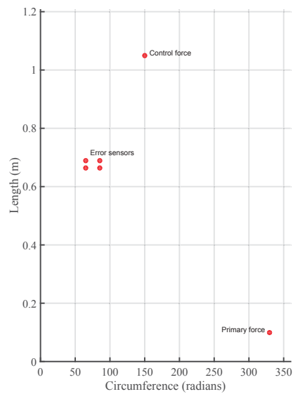
Figure 5.12 Placement of shakers and accelerometers on the shell in configuration B.
