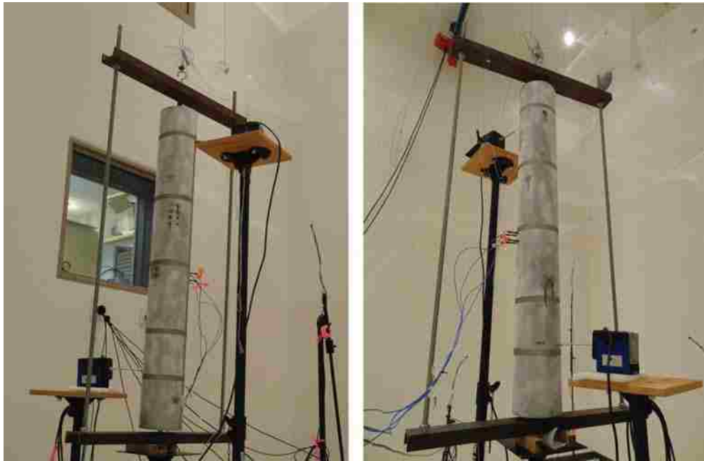
Figure 5.3 The experimental setup showing the mounted cylindrical shell in the frame while the accelerometers and shakers are attached.
