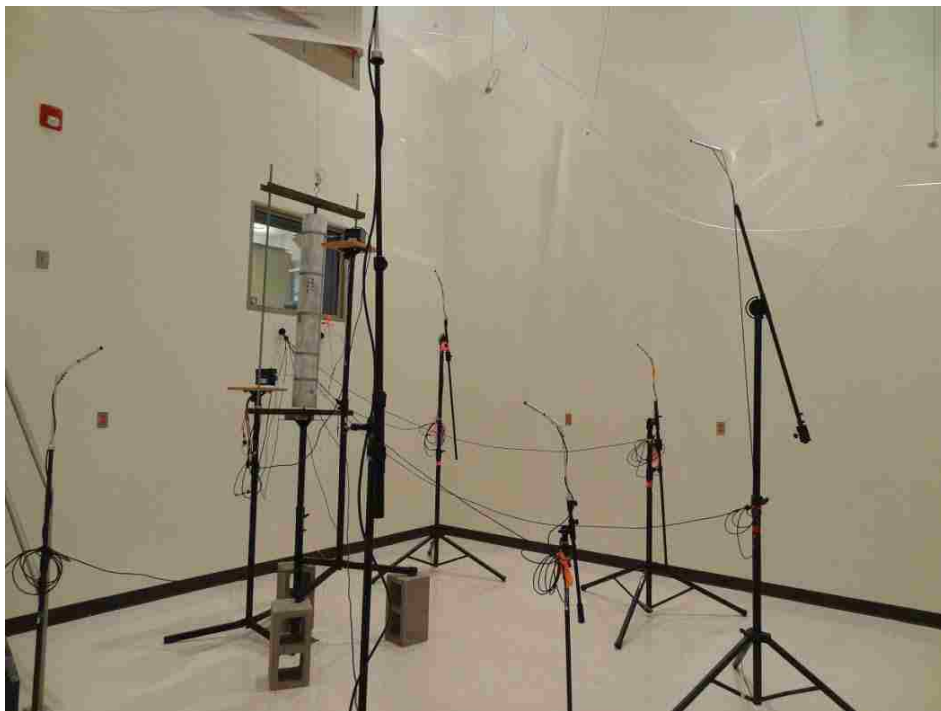
Figure 5.4 The experimental setup showing the cylindrical shell, shakers and accelerometers, as well as the microphone placement.
