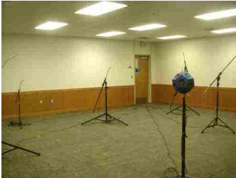
Figure 3.9 The test configuration for determining the frequency-dependent reverberation time of the medium-sized test room. The dodecahedron loudspeaker was excited with a maximum length sequence signal and the impulse response from twelve source-receiver positions were used for averaging, as required by the ISO 354 standard. The average reverberation time was calculated by the integrated impulse response method performed by the EASERA software package.
