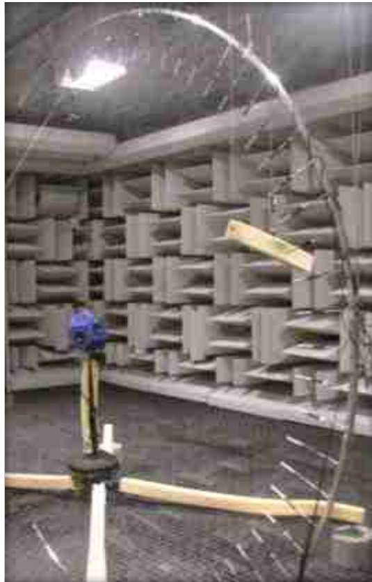
Figure 3.8 The experimental setup for determining the directivity factor and sound power of the source under test in an anechoic chamber. A dodecahedron loudspeaker is shown mounted on a turntable stand. The turntable is covered with absorptive treatment to maintain anechoic conditions. A 180^\circ arc array of 37 microphones senses the radiated field in 5^\circ increments. The source was also rotated in 5^\circ increments in the azimuthal angle.
