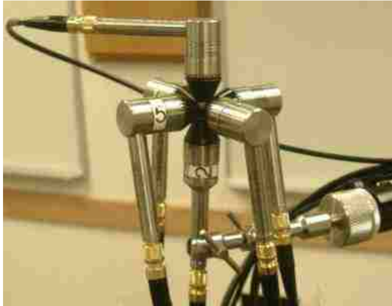
Figure 3.11 View of the G.R.A.S. Type 50VI vector intensity probe.
