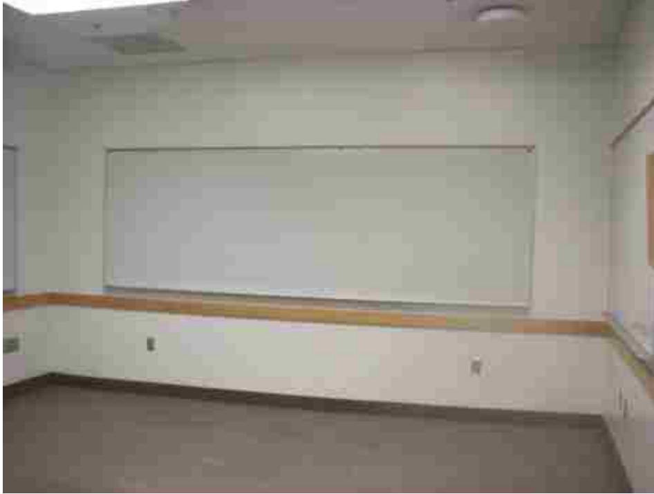
Figure 3.4 A university classroom with dimensions 4.8 x 6.5 x 2.9 m and volume 90.5 m 3 . The floor is carpeted cement, the walls are made of drywall, and the ceiling is composed of suspended acoustic tiling.
