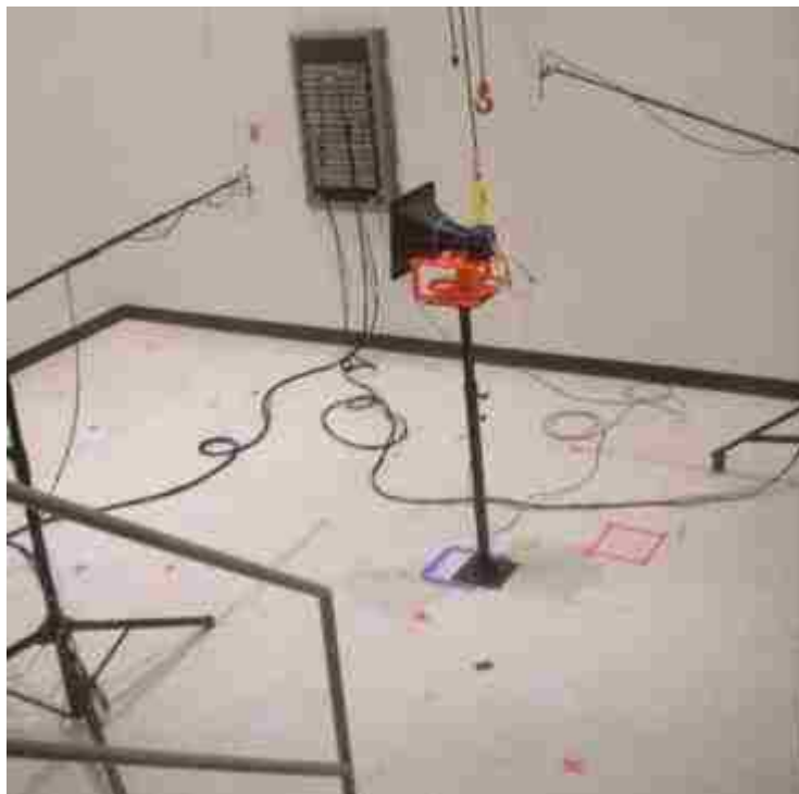
Figure 3.15 ISO 3741 violation test configuration using energy density probes close to the source.
