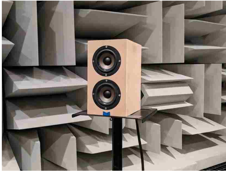
Fig 3.1. The reference directivity source in the anechoic chamber. The lower driver is an active loudspeaker, while the upper driver is a passive radiator.
