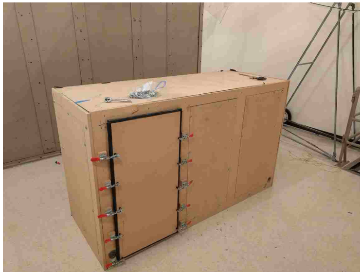
Fig 3.3. The large wooden enclosure assembled in the small reverberation chamber.
