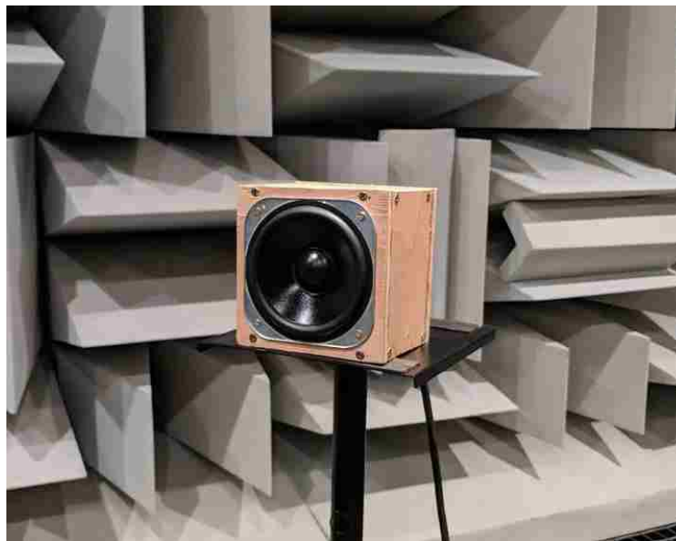
Fig 3.4. The compact source under measurement in the anechoic chamber.
