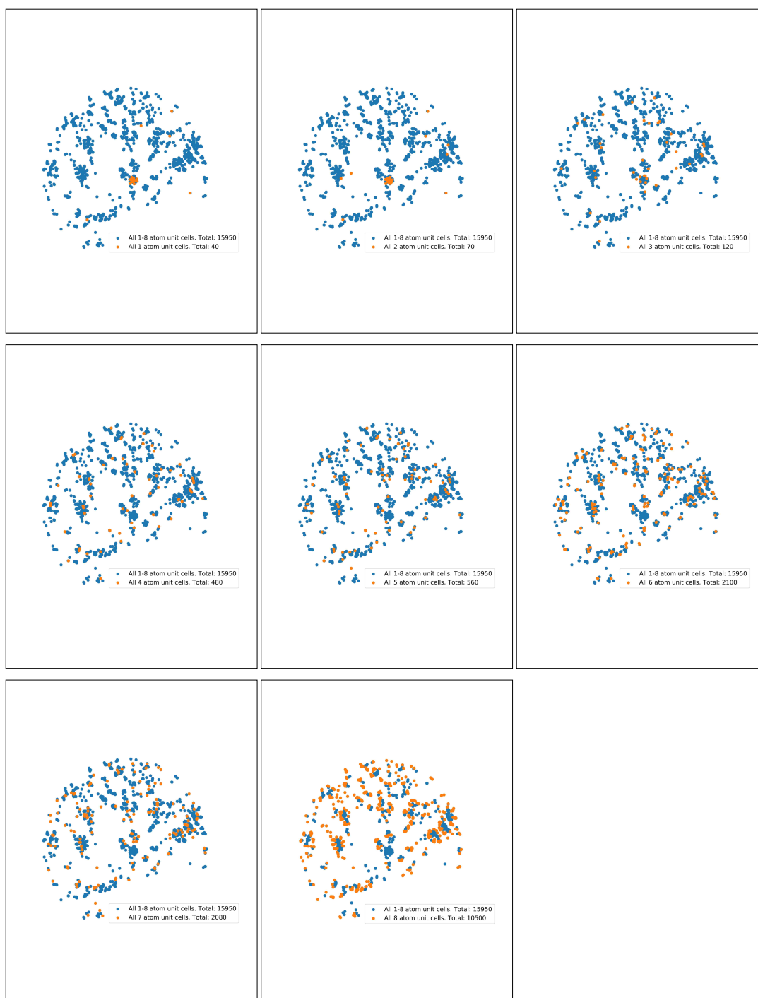
Figure 4. Visualizing all 15950 structures (DFT-10B) using a t-SNE plot. Each structure in the higher-dimensional space (MBTR) is graphically represented on a 2D plane using t-SNE 5 method. We can observe that 1 or 2 atom unit cells are not representative of larger unit cells in the dataset and are away from other higher atom unit cells. This is a possible reason for high prediction errors when 1 or 2 atom cells are not included in the training set.
