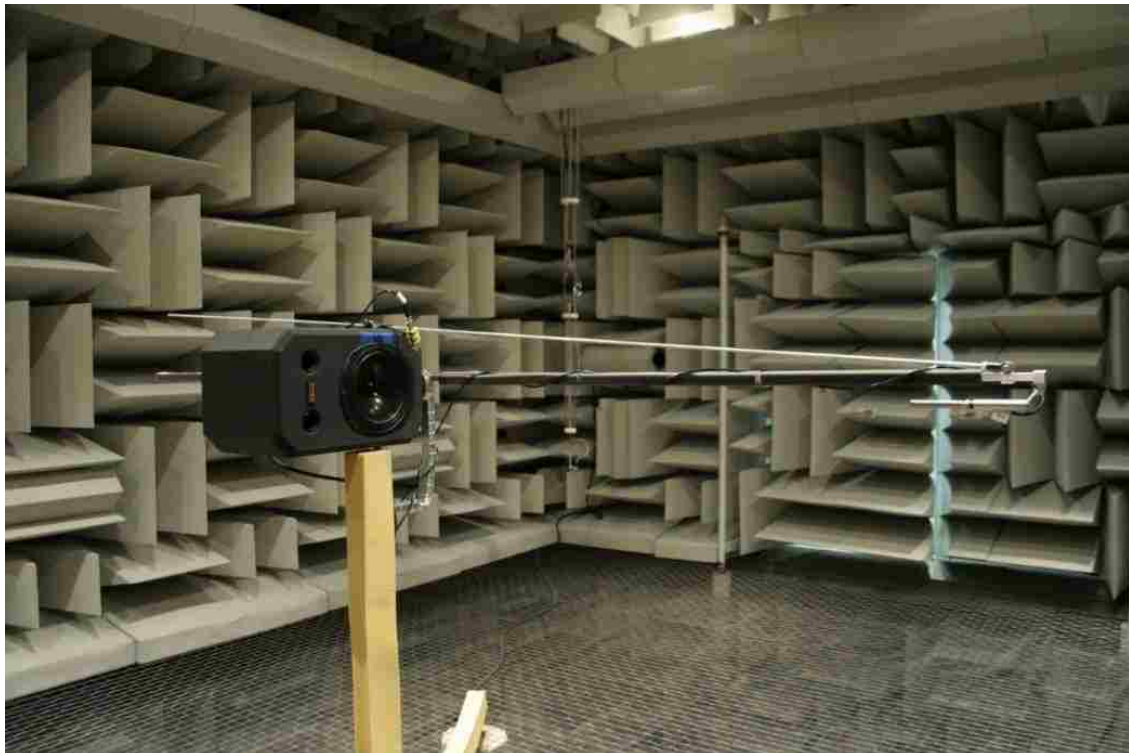
Figure 5.4. Tannoy System 800 loudspeaker outfitted with an adjustable rotating boom arm used to fix a microphone on axis with the loudspeaker, regardless of loudspeaker orientation.
