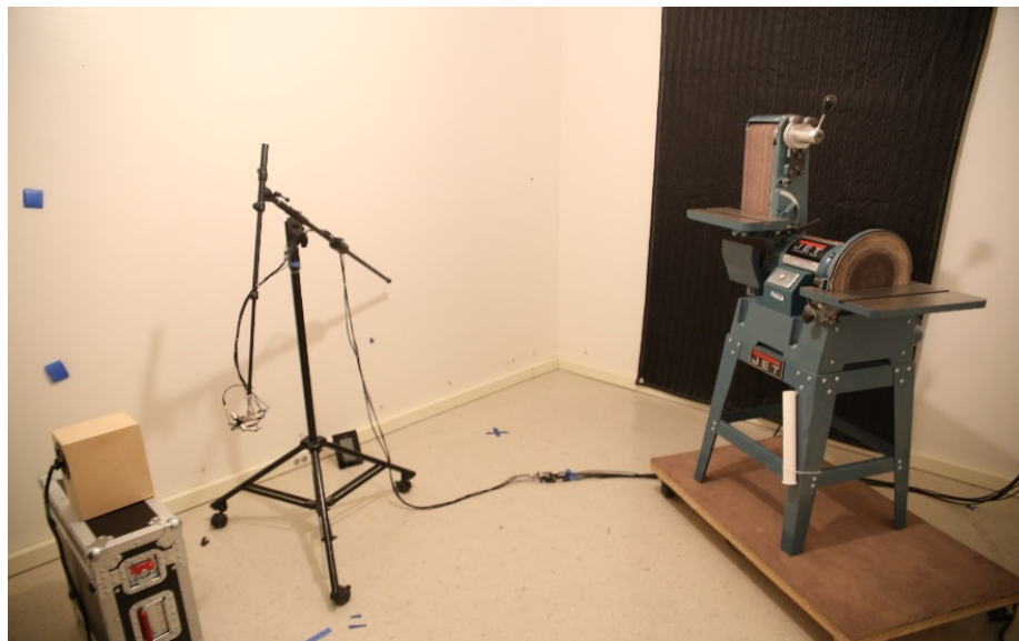
Fig. 4.19. The measurement configuration for the sound power of the belt and disc sander in the VAC with two blankets. The reference directivity source is on the left and the DUT is on the right. The sensor is positioned closer to the former.
