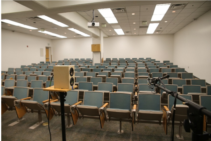
Fig. 4.26. The two-point in situ method in room C215 of the Eyring Science Center on the BYU campus. The reference directivity loudspeaker is shown.
