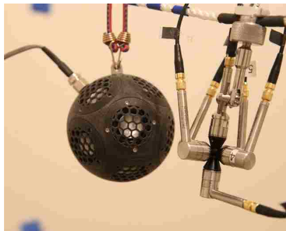
Fig. 4.3. The 7.5 cm spherical dodecahedron loudspeaker and the energy density probe in the VAC.
