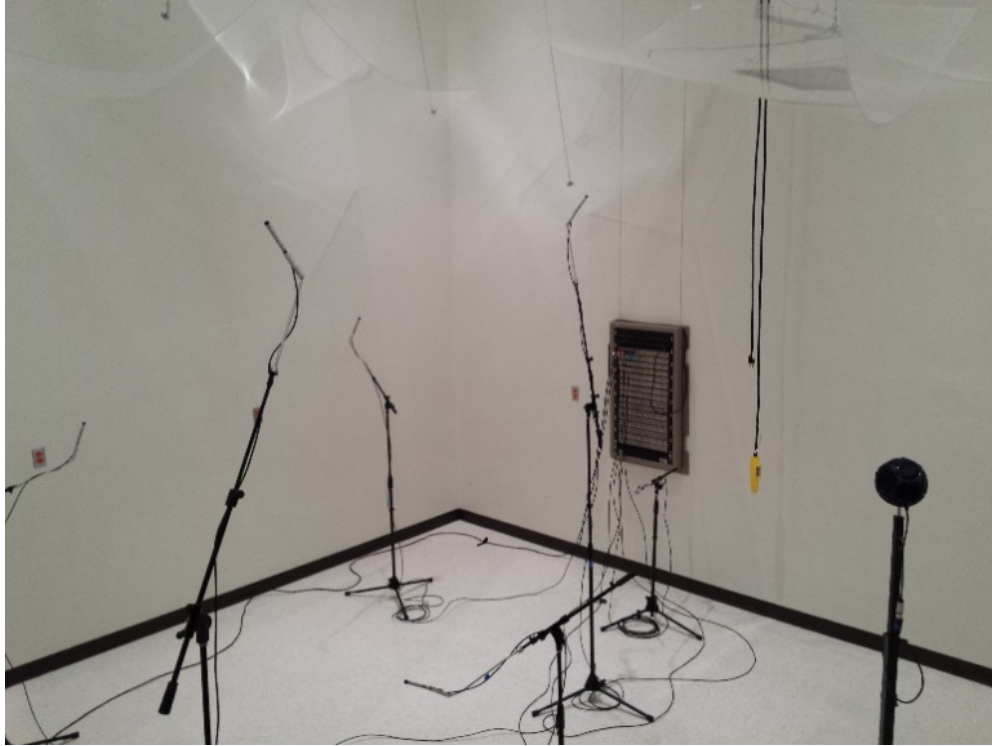
Fig. C.2. A setup in the reverberation chamber for ISO 3741, including six microphones. Several clear diffusers in the reverberation chamber are also pictured hanging from the ceiling.
