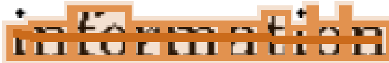
Figure 88 The highlighter stroke (dark brown) using the leaf intersection algorithm has missed the dots in the 'i's.
