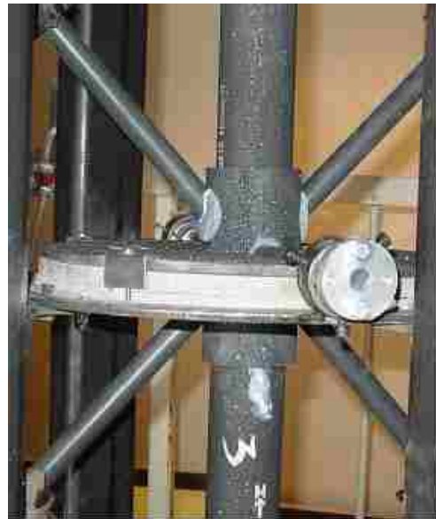
Figure 14: Windows section showing inner reactor tube with optical access; before applying insulation material
