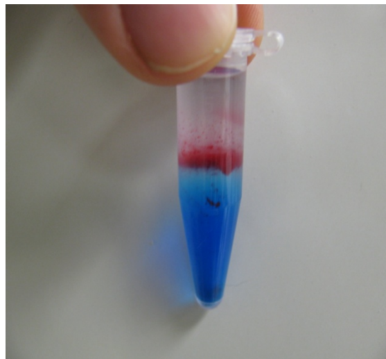
Figure 8: Pillow density method. Top layer (clear) contains sodium chloride. Bottom layer (blue) contains sucrose. Middle layer (red) contains eLiposomes. This is a two-layer pillow density technique.
