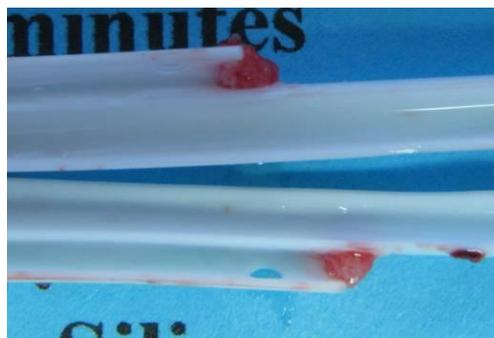
**Figure 8.9. Late thrombus growth in second Mahurkar catheter. Thrombus has only occluded the main inlet port. (Run time = 40 min.)**
