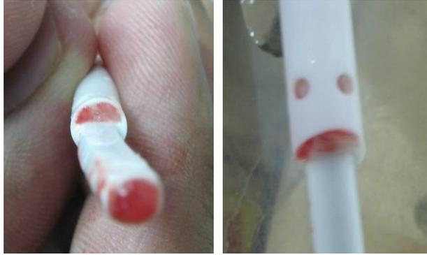
**Figure 8.7. Early thrombus growth in first Mahurkar catheter. The occlusion of the main port can clearly be seen in the left-hand image, whereas the side ports are still clear of thrombus in the right-hand image. (Run time = 12 min.)**
