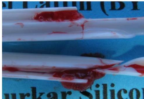
**Figure 8.8. Late thrombus growth in first Mahurkar catheter. Near-total occlusion of both the main and side inlet ports is visible. (Run time = 27 min.)**
