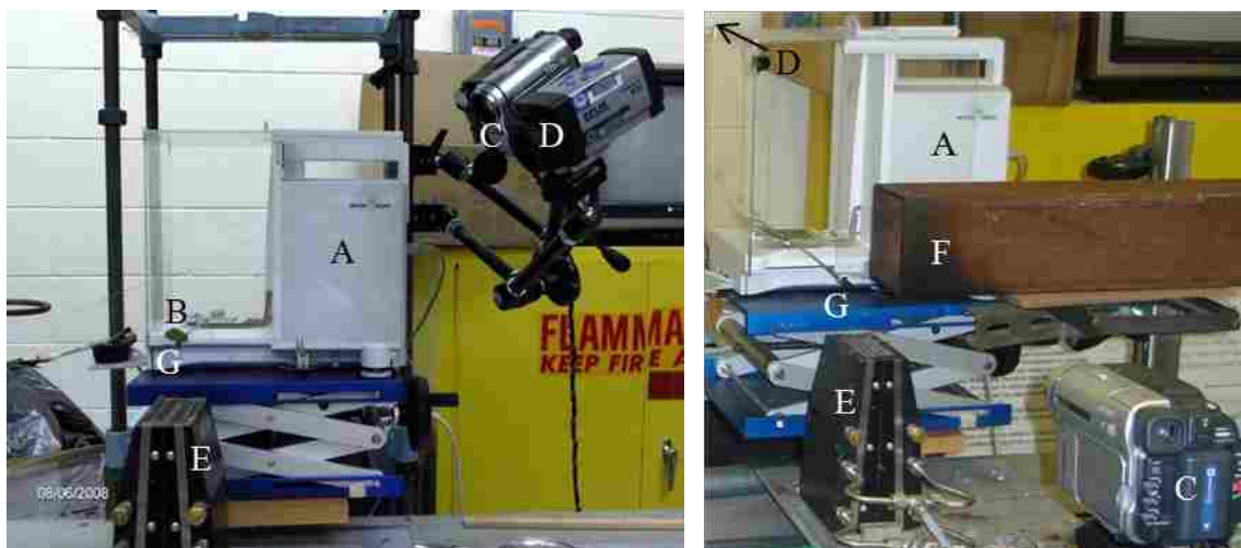
Figure 4-2. The experimental apparatus is shown configured for no wind (left) and wind-blown (right) experiments. A mass balance (A), leaf (B), video camera (C), IR camera (D), flat-flame burner on movable cart (E), square duct with fan and honeycomb mesh (F), and an alligator clip for holding fuel samples (G) are identified.
