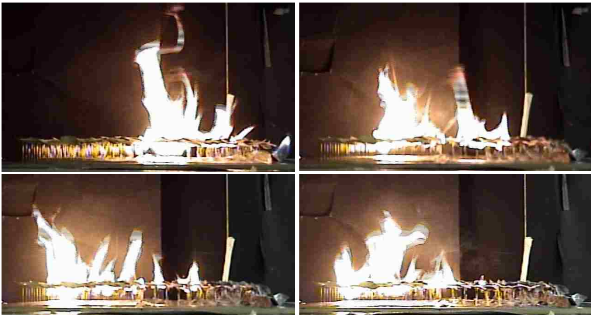
Figure E-10. Skewered leaf Experiment 2 showing flame extension below the leaf surface while fire crosses the 1.5 cm gap.
