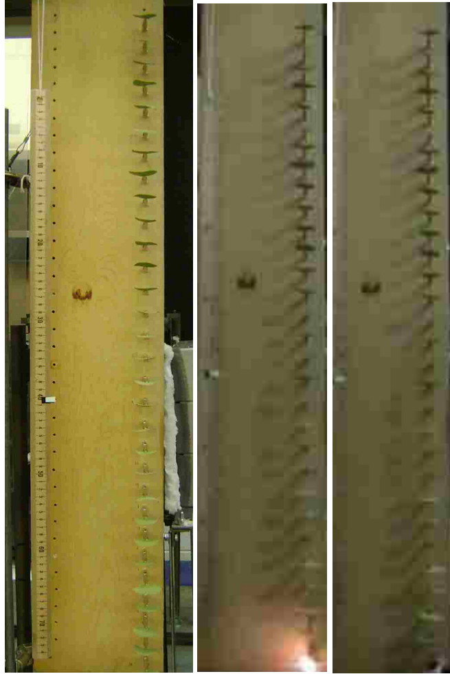
Figure E-1. Horizontally-oriented leaves in a vertical column. Left: prior to flame contact. Center: at start of heating (0 s). Right: at burn out (26 s).
