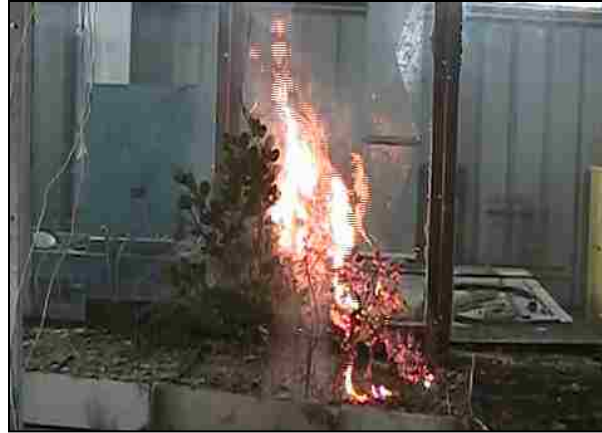
Figure A-14. Manzanita combustion experiment from December 2009, mixing branches with 10% and 30 % moisture content. The flame shown here burned out shortly after this time, leaving the 10% moisture content side of the bush burned and the 30% moisture content side unburned.
