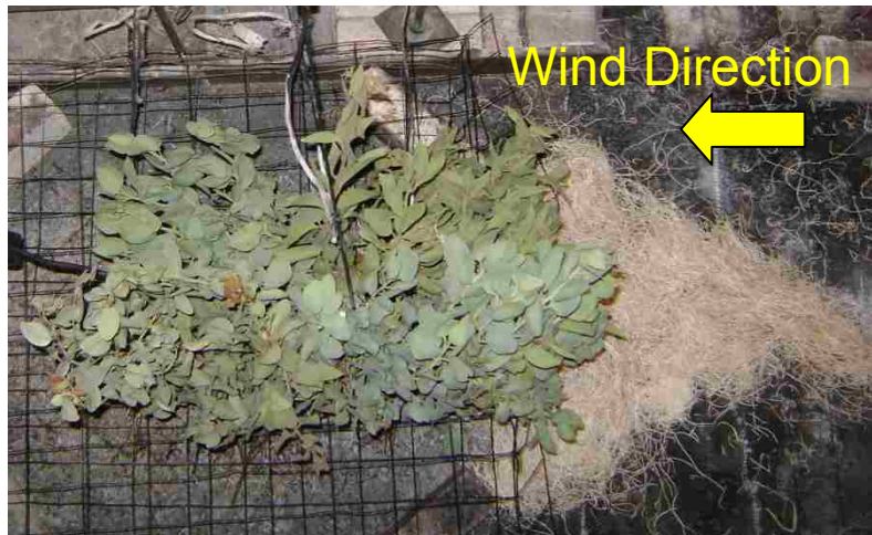
Figure A-1. Top view of the setup of an experiment with manzanita and zero wind speed. Note how the v-shaped bed of excelsior is in contact with the branches.
