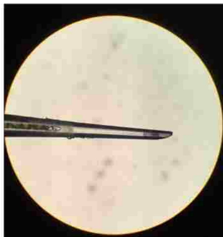
Supplemental Figure S1. Column with integrated electropray tip. (A) Column packed with 1.7 \mu\text{m} C18 and (B) pulled electropray tip.
