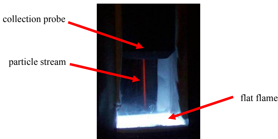
Figure 5.2. Biomass particles being pyrolyzed in the FFB reactor at the T_{gas,max} = 1433 K condition.
