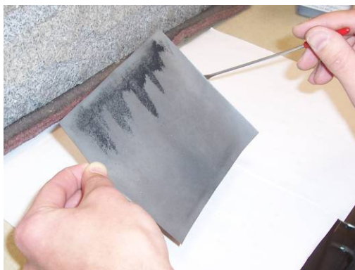
Figure 4.10. Separating char by shape using an inclined piece of 600-grit sandpaper.
