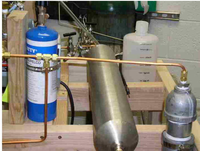
Figure 23. Ballast tank, V-101.
