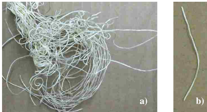
Figure 4.14. Excelsior samples as (a) grouped bands or strings and as (b) arbitrary length used for experimental run.
