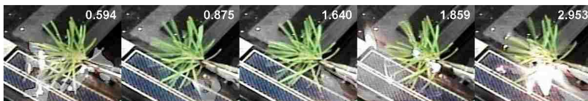
Figure 5.2. Jetting sequence for a Douglas-fir sample. Numbers indicate the time difference (s) from the initial time of the experimental run. Video in Appendix D.
