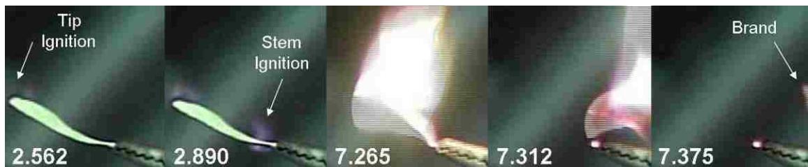
Figure 5.12. Brand formation sequence of sagebrush leaf showing tip and stem ignition as well as leaf brand. Numbers indicate the time difference (s) from the initial time of the experimental run. Video in Appendix D.
