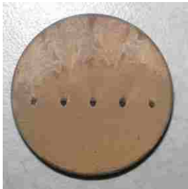
Figure 4.7 Cylindrical holes coupon with a) 3.75 mm spacing (M3), b) 4.5 mm spacing(M4)
