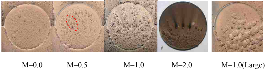
Figure 5.26 Variation of deposit patterns from fine particles and large particle (right side) on the M3 coupon surface with hole spacing 3.375d at blowing ratios from M = 0 to M = 2.0 (holes 1 & 5 blocked)
