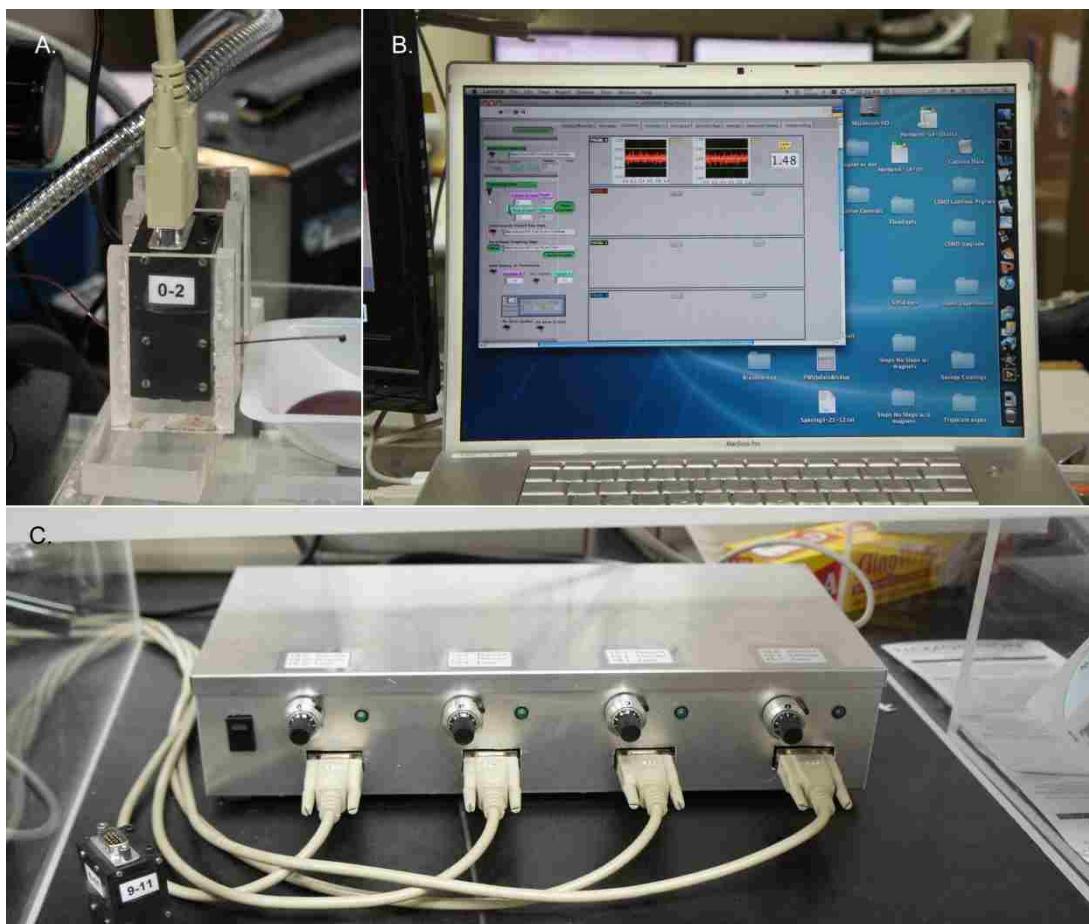
Figure 13: A) Laser Cuvette B) LabView® C) LSMD Controller.
