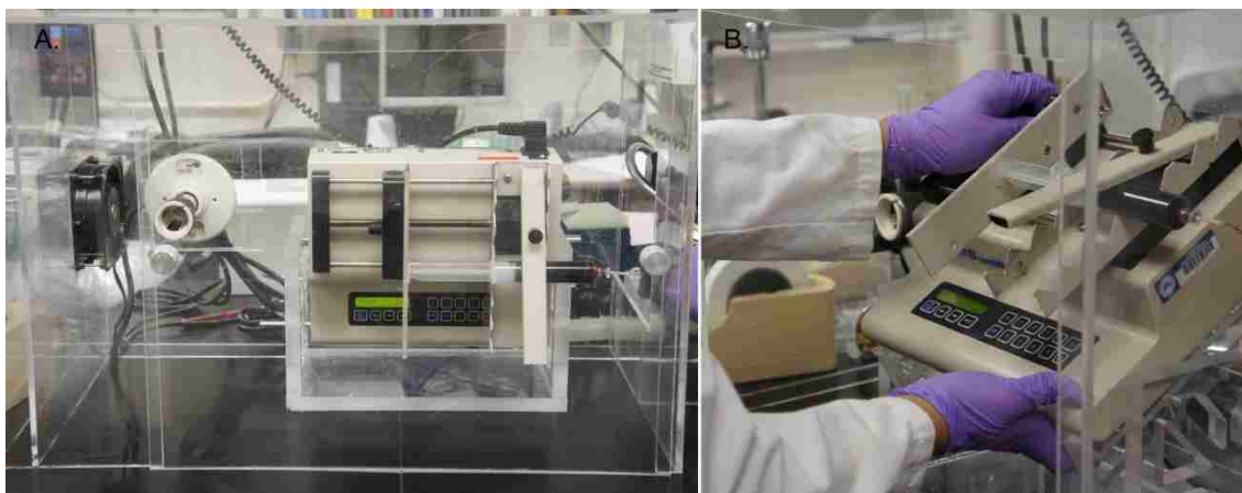
Figure 11: A) Syringe pump set-up B) Syringe pump rotation.
