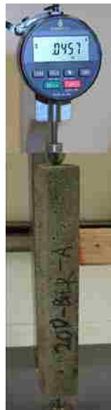
Figure 4-10 ASR bar length measurement (precision \pm 10^{-4} in)
