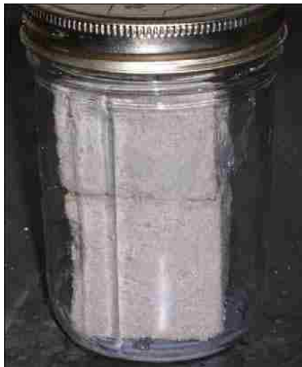
Figure 4-6 Vacuum and moisture curing of 2 in cube samples
