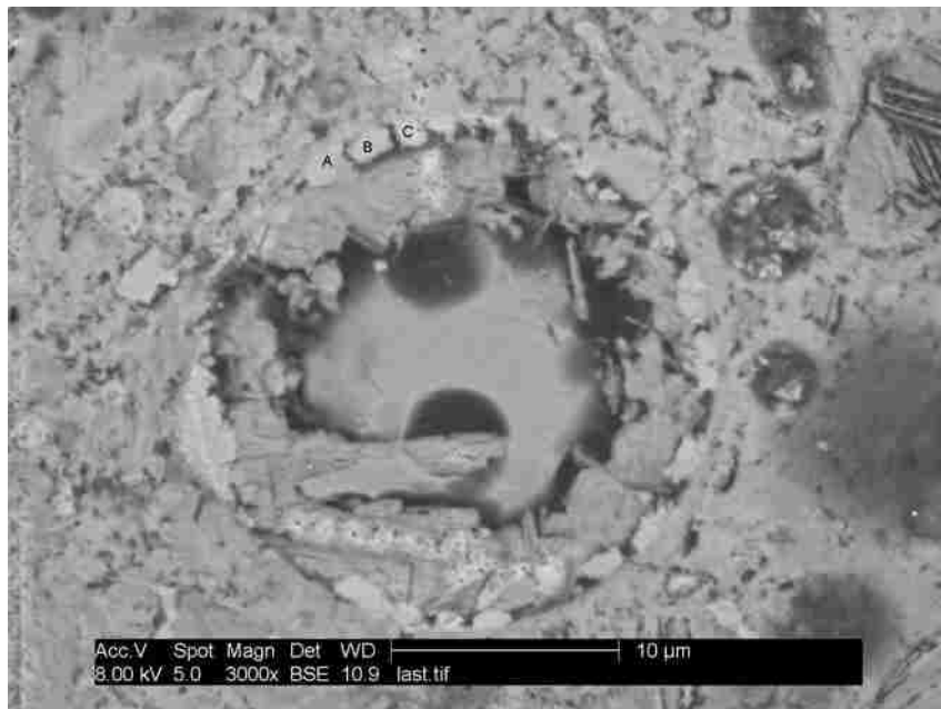
Figure 5-15 Reactive class C fly ash particle at one year of curing
