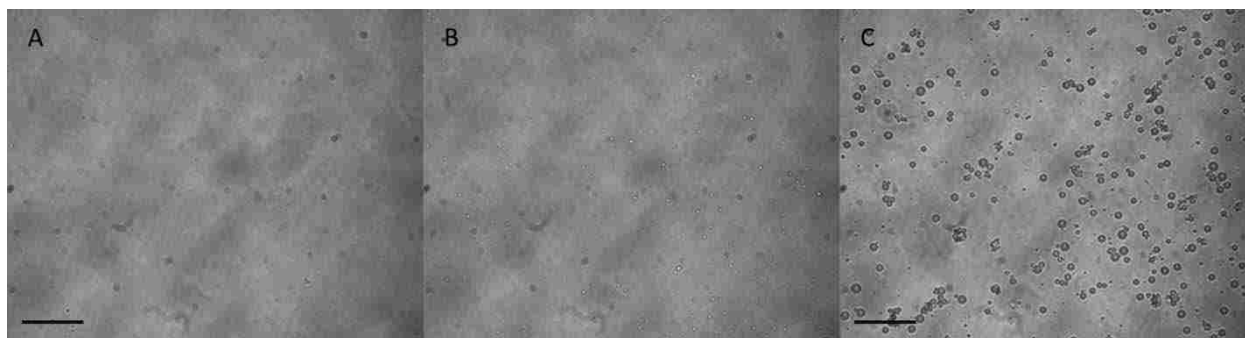
Figure 14. Small PFC5 emulsion before heating (A) and before (B) and after (C) ultrasound exposure at 37°C. The microscope slide was heated to 37°C and 20-kHz ultrasound was applied for 5 seconds at 1 W/cm 2 . Heating had no significant effect on the appearance of the emulsion (A and B). After ultrasound exposure, droplets had vaporized and coalesced into much larger bubbles (B). However, these bubbles were less prominent than those formed from large PFC5 droplets. Scale bars represent 50 μm.
