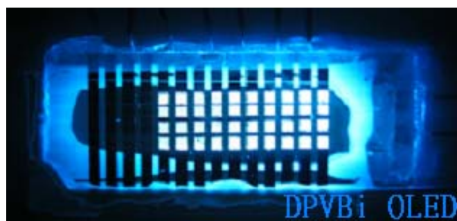
Figure 3. A 4 \times 14 array of blue DPVBi OLEDs used to excite the PL of the reaction product of ADA and hydrazine. In the image at right, 4 \times 10 pixels are lit. Each pixel is \sim 2 \times 2 \text{ mm}^2 .
