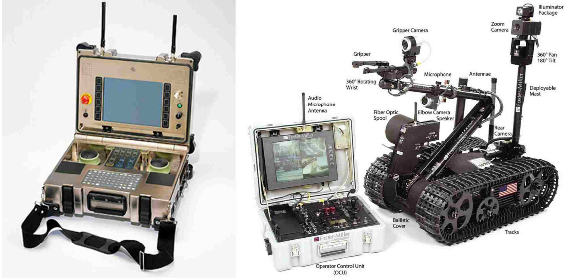
Figure 1.4: Left: iRobot Packbot OCU. Right: Foster-Miller Talon mobile manipulation robot and OCU.
