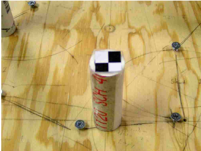
Figure 3.2: Closeup of stereo camera calibration target.
