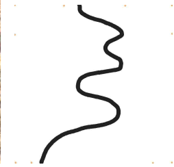
Figure 4.2: Mountain pass created with 10 fixed points and a single road feature stroke.
