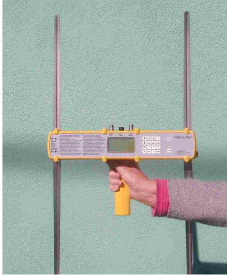
Figure 3.2: The Little L-Per from L-Tronics. This is an example of a dual-dipole type homing RDF unit.
