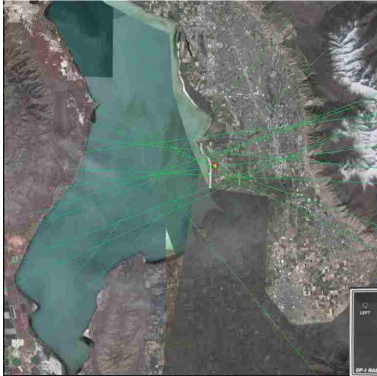
Figure 4.2: Visualization of the Lake Dataset. Locations of the readings are shown on the left side of the map and the bearings are represented by the lines. The icon on the right side of the map approximates the known location of the transmitter (shown only for reference).
