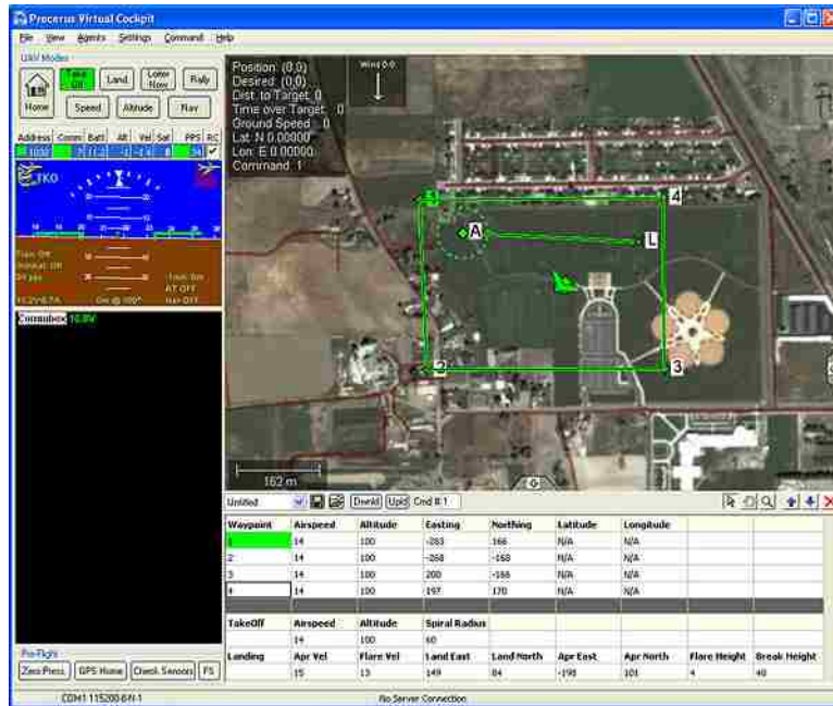
Figure 3.1: The Virtual Cockpit program. This constitutes BYU groundstation control.
