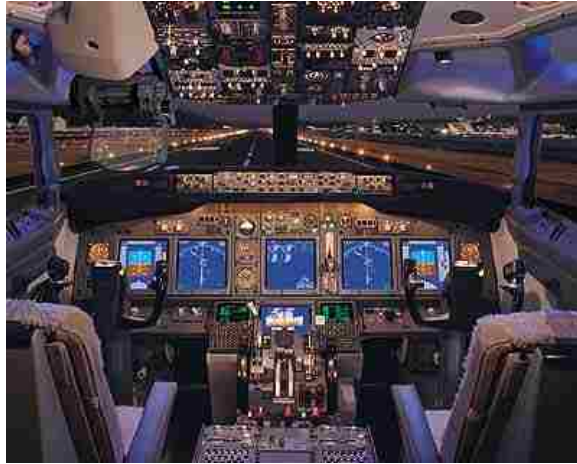
Figure 2.4: Boeing business jet glass-cockpit (from http://www.b737.org.uk )
