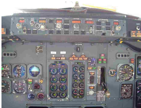
Figure 2.2: Boeing 737 center panel (from http://www.b737.org.uk )
