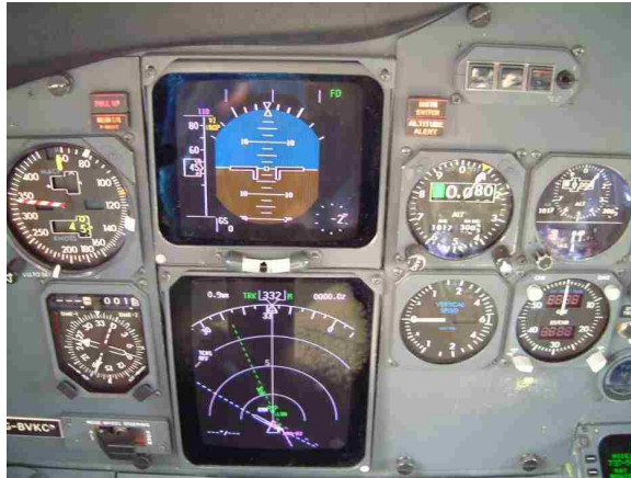
Figure 2.1: Boeing 737 captain's instruments (from http://www.b737.org.uk )
