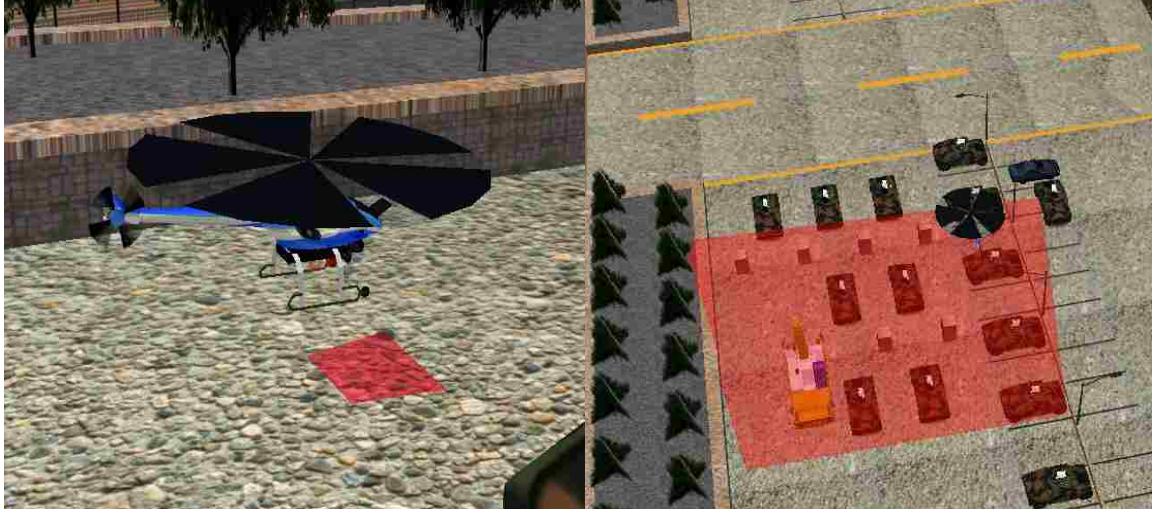
Figure 4.1: The decreasing field of view as the aircraft nears the ground will restrict its movement greatly. In the figure on the right, the aircraft hovers high above an obstacle field (in simulation). The aircraft can track any landing site in the red-highlighted field of view. In the figure on the left, the aircraft has selected the landing site north of the crane. Now that the aircraft is near the ground, very little motion in the field of view is possible before the target is out of sight.
