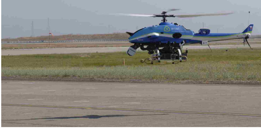
Figure 2.1: The ARP project operates a Yamaha R-MAX UAV platform with a high-precision digital IMU, differential GPS, ground height measurements from radar, sonar, and laser, weight-on-wheels switches, and digital cameras for navigation by machine vision algorithms.
