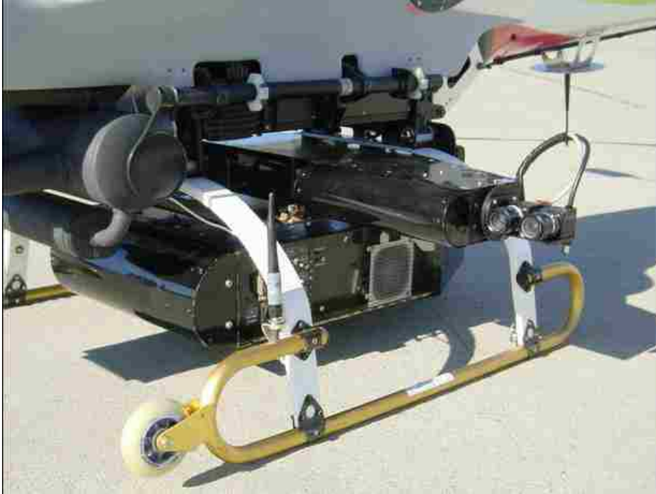
Figure 3.1: The ARP left and color camera are mounted on the left end of the payload. The right stereo camera is mounted on the opposite side.
