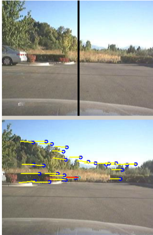
Figure 27 - Example of using interesting points to track movement Point match movement vectors are shown with blue circles (interesting point from previous image) with yellow lines (movement since previous image). The overall movement that was calculated is shown with a green circle and a red line.
