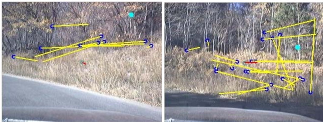
Figure 33 - Close Grass confuses Interesting Point matching These are two examples of the Interesting Point matching algorithm failing with close uniform objects
