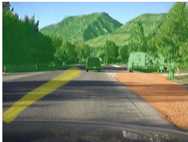
Figure 1 - Different Obstacle Types Flat (Yellow) – Lane markers; Negative (Orange) – Lower Shoulder; Positive (Green) – Trees, Other Vehicles, Homes
