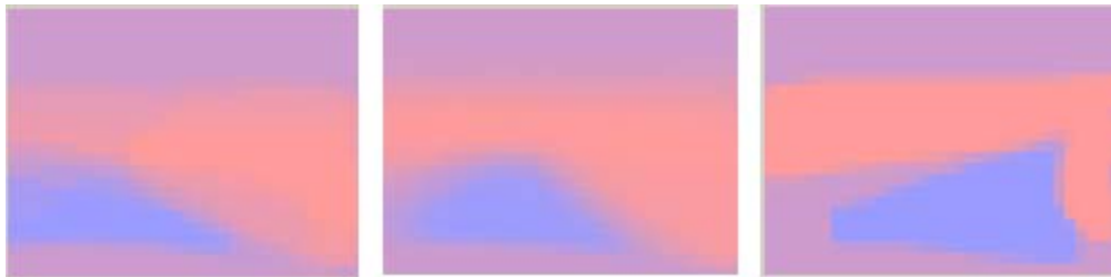
Figure 36 - Sample Probability Grids Red represents obstacles, Blue represents safe areas, Blends (shades of purple) represent varying degrees of certainty; Left is from Left Turns, Center is from Straight Movement, Right is from Right Turns
