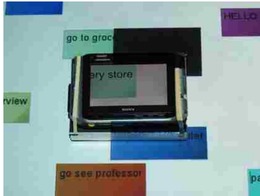
Figure 36 Synchronization between handheld and DiamondTouch table
