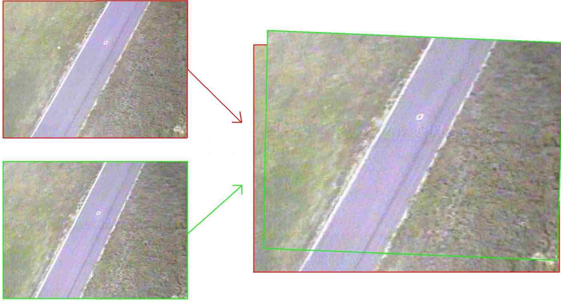
Figure 2.1: An example of two frames (left) that have been spatially aligned into one image (right) after being registered to each other. The image on the right is the aggregation or mosaic of the two frames on the left.
