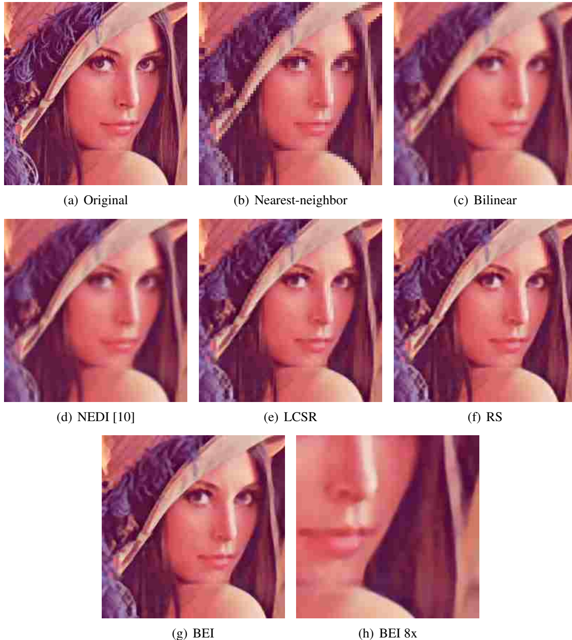
Figure 3.9: A 256 \times 256 region of “Lena” (a) decimated twice and magnified 4x (b – g). Note the gradient steps in (e) and (f), especially in steep gradients such as on the nose and in the shadow on the forehead. Because BEI can model decimation blur explicitly in the capture and recapture processes, it preserves these gradients at 4x (g) and 8x (h) while keeping boundaries sharp.
