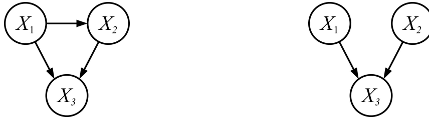
(a) A directed acyclic graph (DAG) that represents the decomposition P(X_1) P(X_2|X_1) P(X_3|X_1, X_2) .
