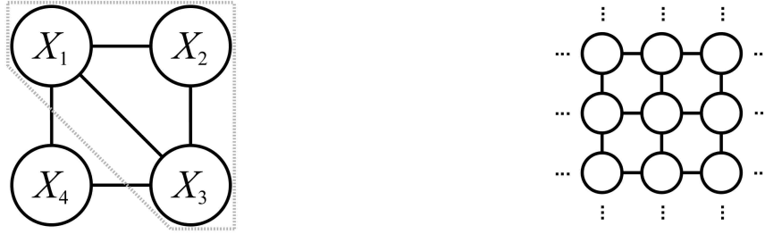
(a) A simple Markov random field with two cliques: \{X_1, X_2, X_3\} (indicated) and \{X_1, X_3, X_4\} . These have associated clique potentials \Phi_1(x_1, x_2, x_3) and \Phi_2(x_1, x_3, x_4) .
