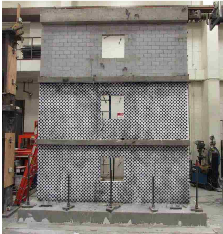
Figure 3-2: Completed wall prior to testing
