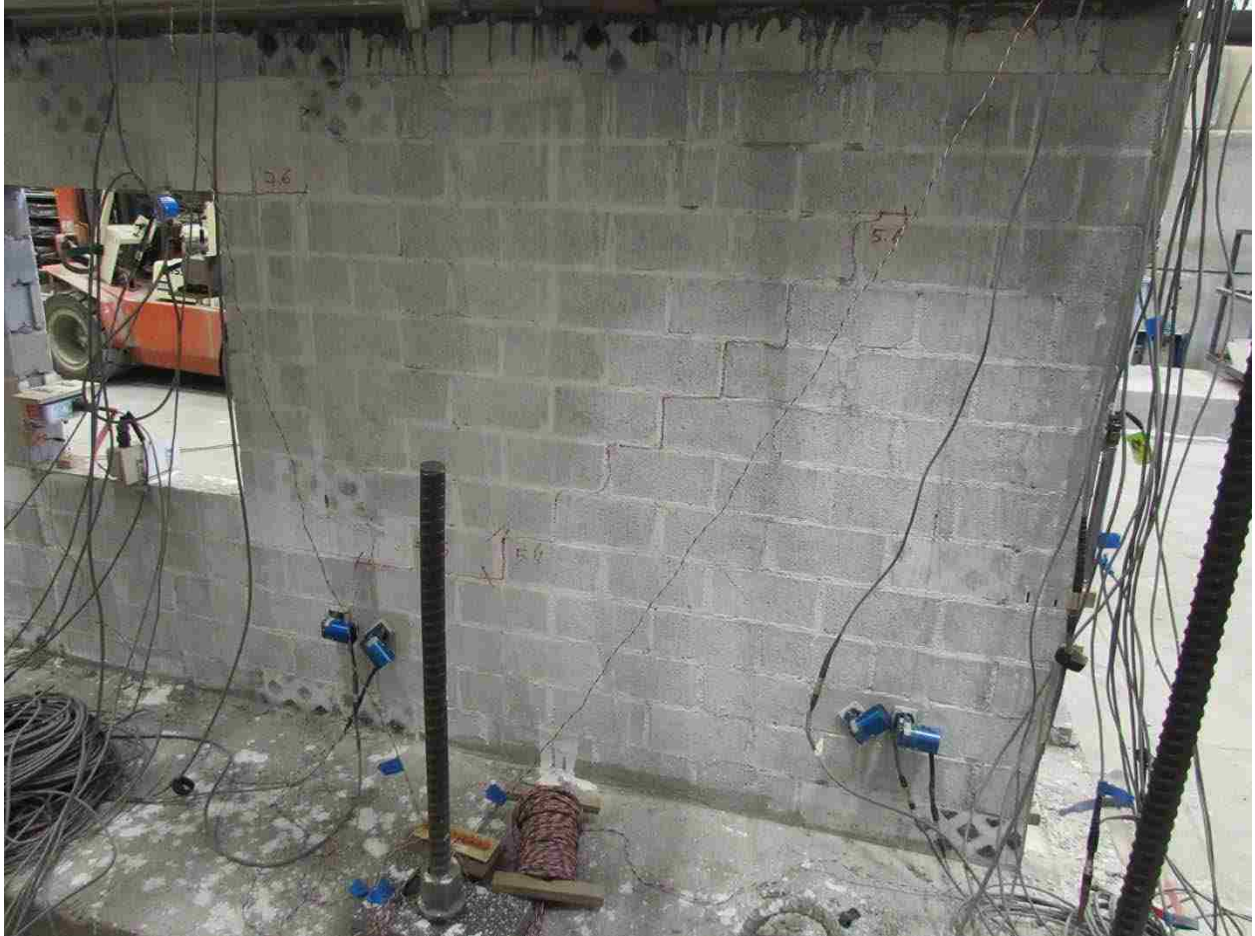
Figure C-2: Enlarged view of 1 st story cracks in pull regime
