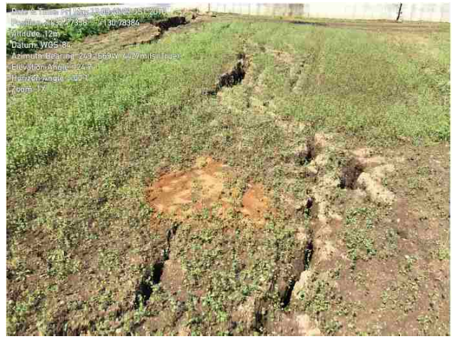
Figure 6-26. Hypothesized lateral spread at site 4 and observed fissures and ejecta (Kayen et al., 2017)
