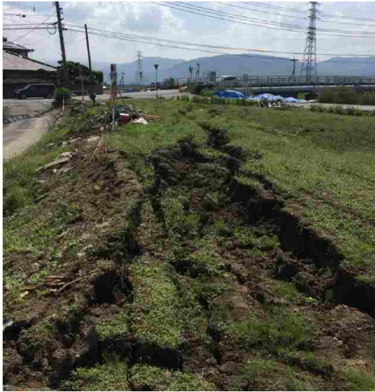
Figure 6-26. Hypothesized lateral spread at site 4 and observed fissures and ejecta (Kayen et al., 2017)
