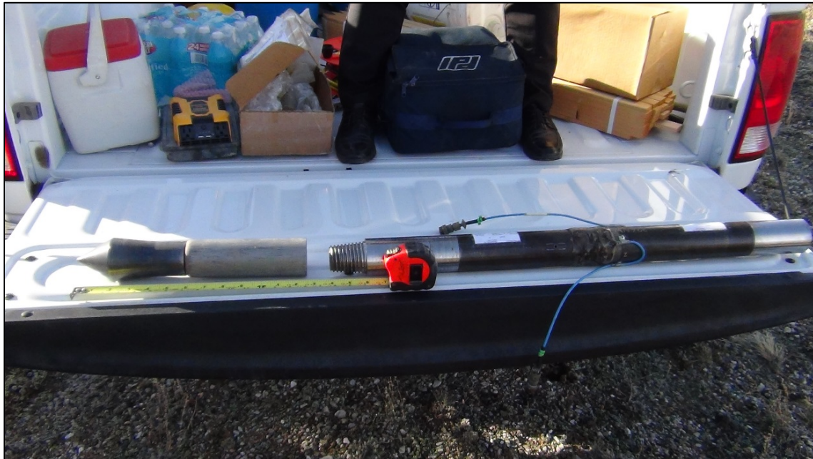
Figure 7-4. View of cone tip, thread adapter, and PDA rod section.
