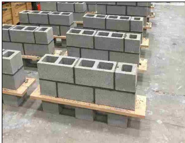
Figure 12. Wallettes Prior to Grouting
