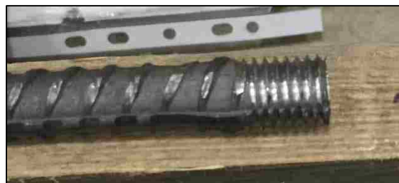
Figure 7. Typical Upset Threads
