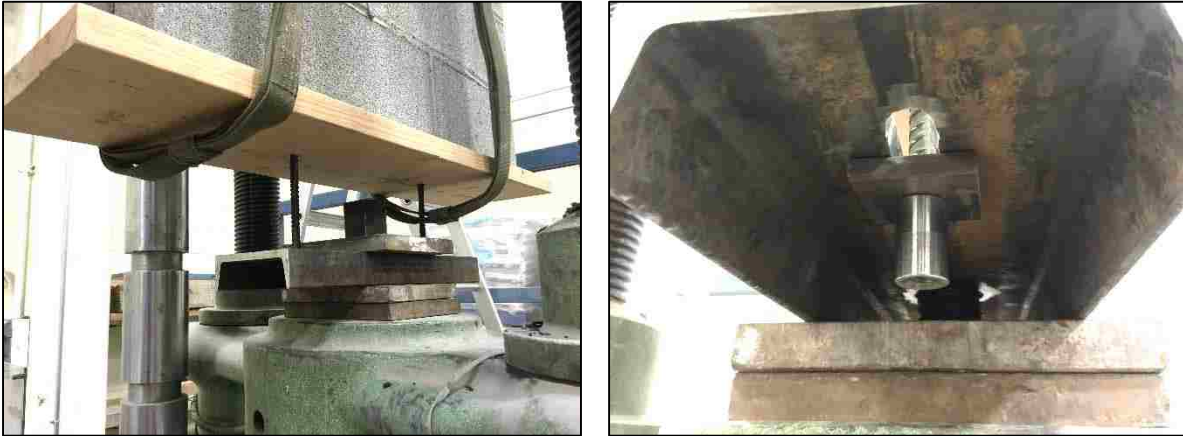
Figure 27. Connection of the Wallette Specimen to the Test Frame
