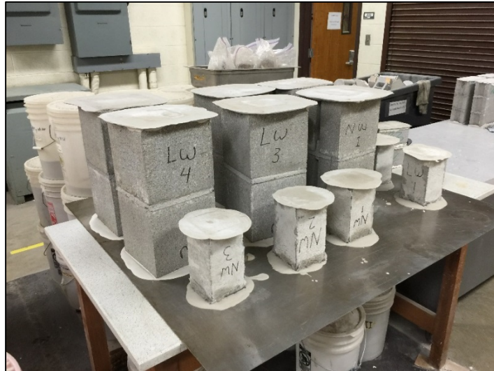
Figure 23. Capping of Grout and Masonry Prisms
