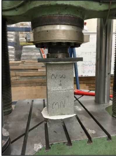
Figure 24. Test Setup for Grout and Masonry Prisms
