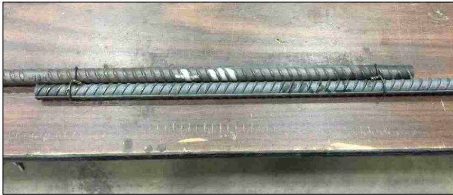
Figure 14. Typical Reinforcement Splice
