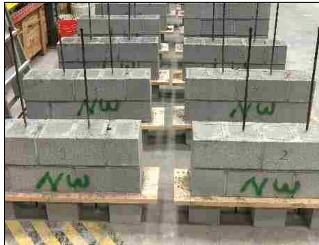
Figure 21. Completed Wallettes Prior to Testing
