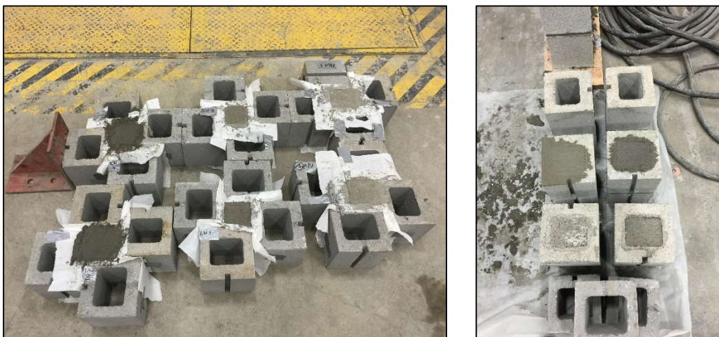
Figure 20. Grout and Masonry Prisms
