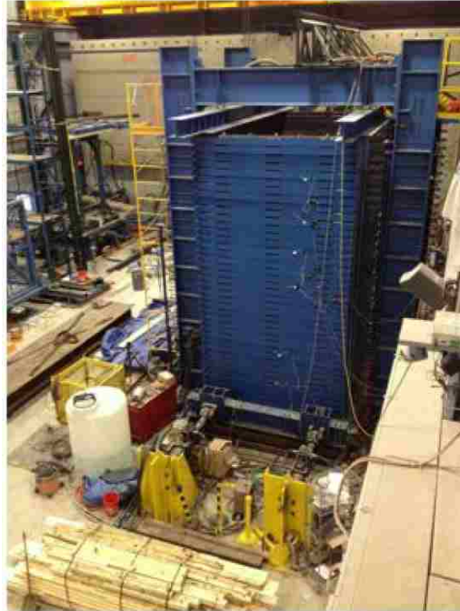
Figure 3-2: Actuators Placed against the Laminar Shear Boxes
