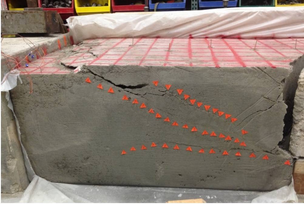
Figure 4-12. Highlighted failure planes.
