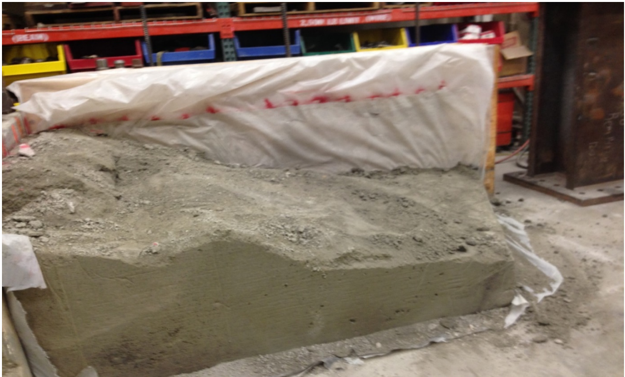
Figure 4-14. Photograph of the three-dimensional failure surface from the south side.
