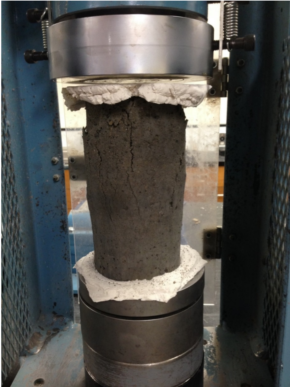
Figure 3-8. Gypsum Cement capped CLSM cylinder after failure.
