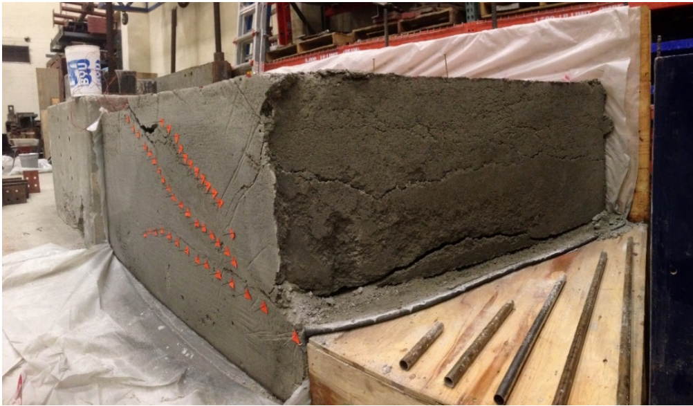
Figure 4-13. Isometric view of the failure planes.
