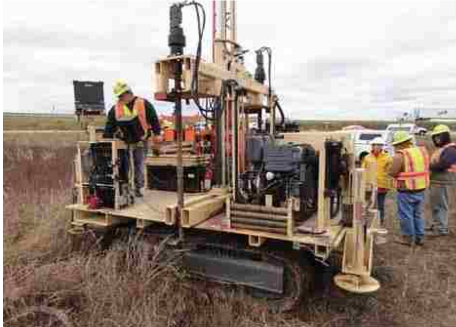
Figure 3.1-4 Photo the Missouri Department of Transportation cone penetration Test (CPT) rig (Bey 2014).
