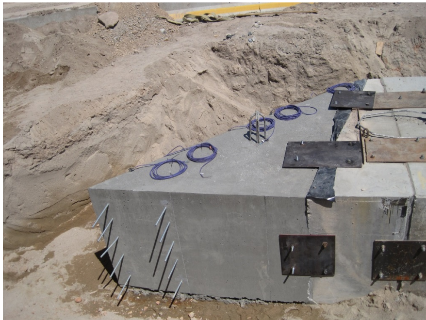
Figure 3-7: Photo of 45 Degree Concrete Wedge with Plates to Ensure Rigid Movement
