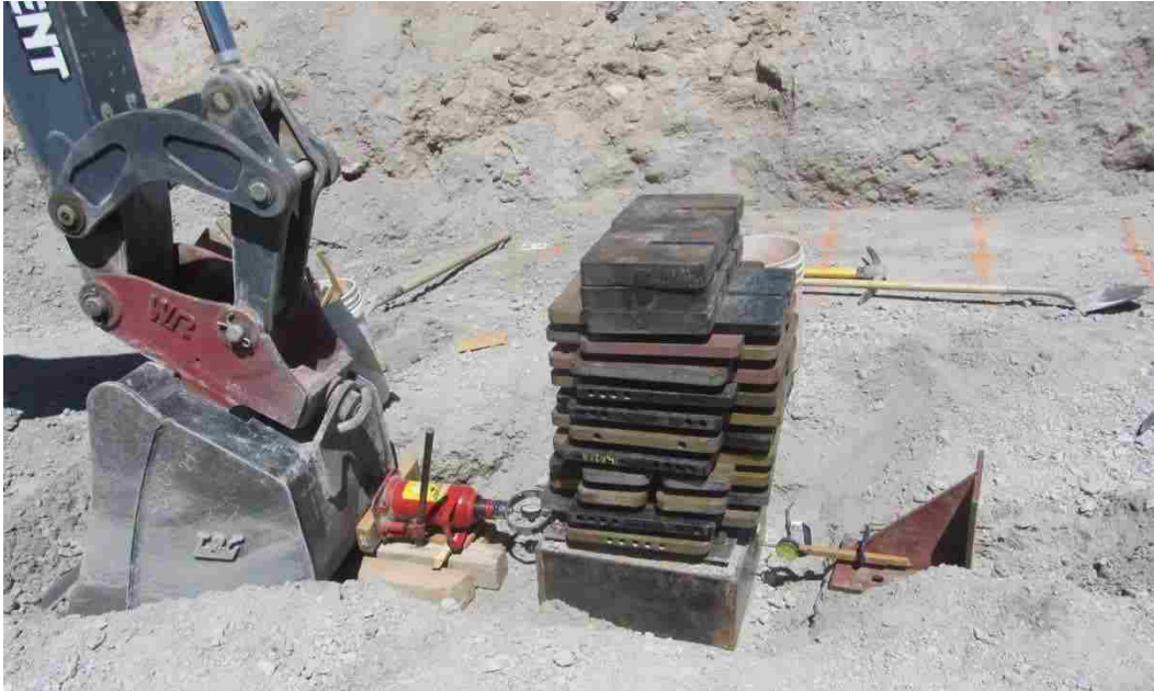
Figure 3-14: In-situ Direct Shear Test Setup.
