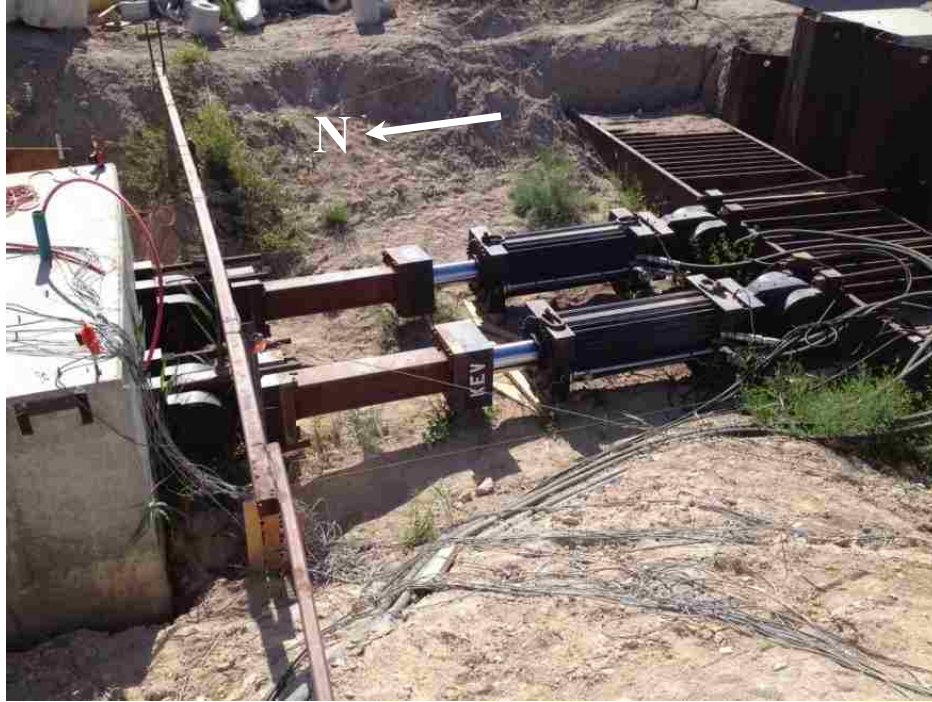
Figure 3-6. Two 600-kip actuators comprised the loading apparatus.
