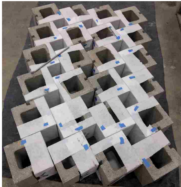
Figure 3-1: Grout Prism Molds
