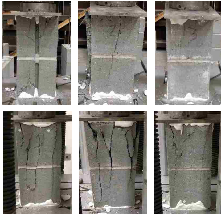
Figure C-4: SCG Prisms at 32-Day Failure
