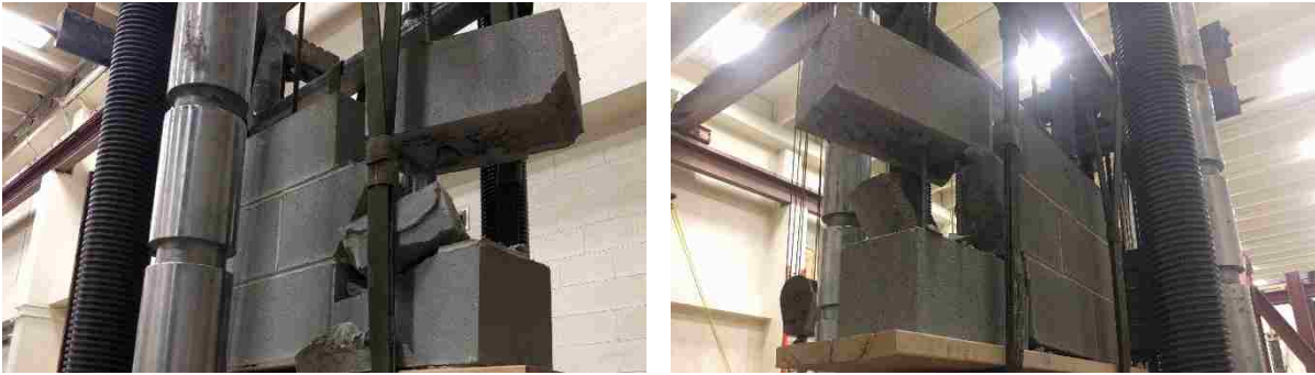
Figure C-11: Test Group 2 Masonry Panel C at Failure
