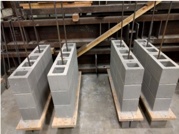
Figure 3-5: Panels Before Grouting
