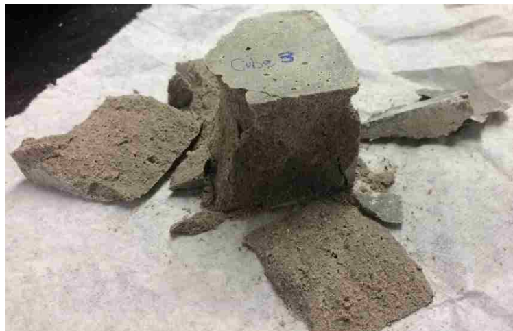
Figure 3-12: Mortar Cube After Compression Testing
