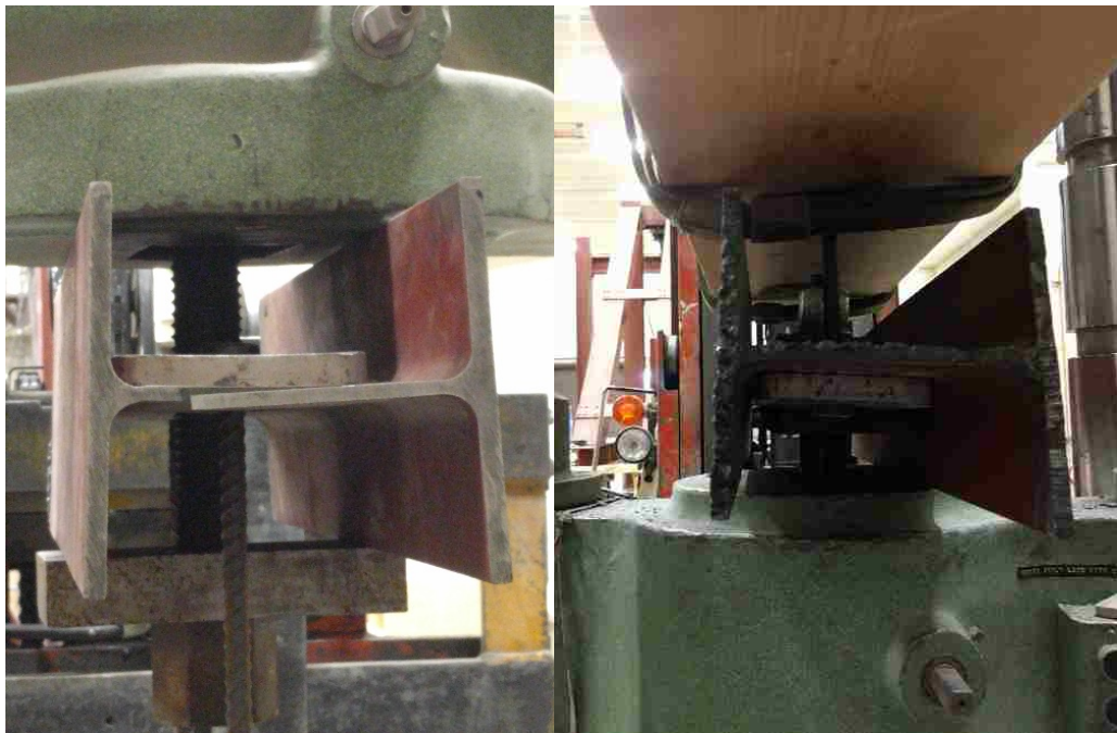
Figure 3-18: Headed Rebar to Test Frame Connections
