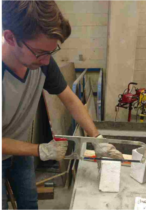
Figure 4-3 : Extraction of cellular concrete cylinders as per Elastizell recommendations.
