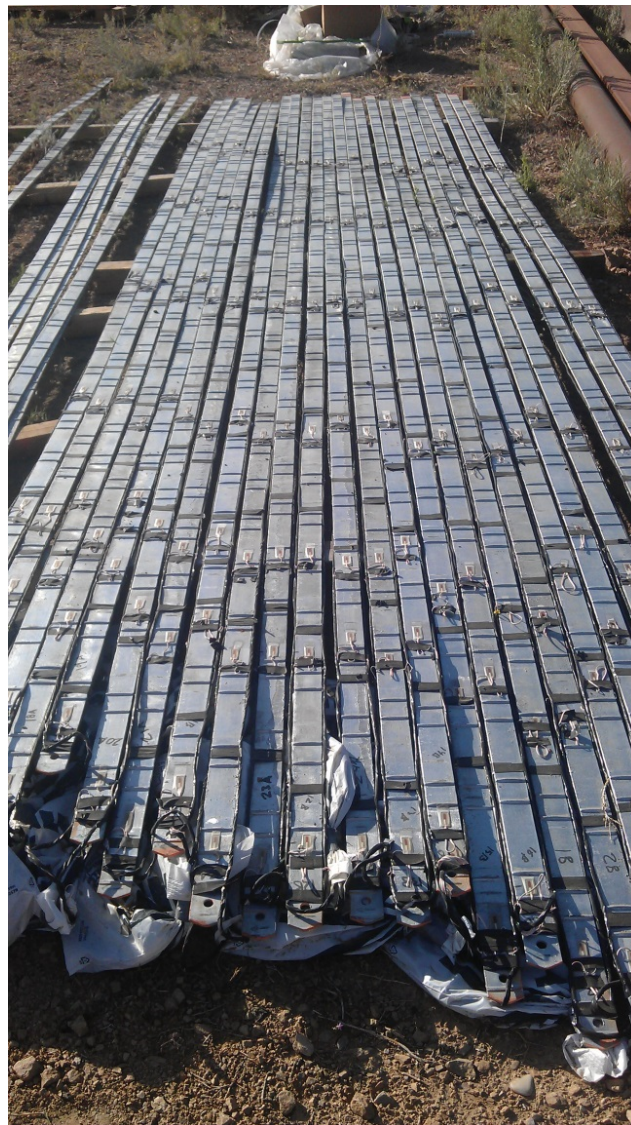
Figure 4-1: Several instrumented soil reinforcement strips.
