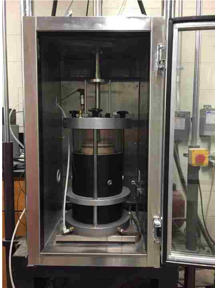
Figure 3-9: Triaxial cell placed inside the UTM-100.
