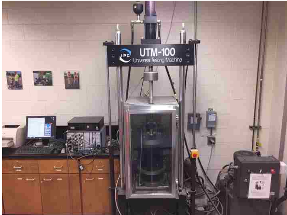
Figure 3-6: UTM-100 testing equipment.
